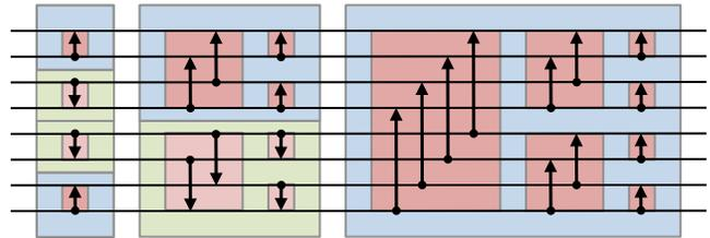
**Figure 4.** Bitonic sorting network of size 8. Adapted from <https://commons.wikimedia.org/wiki/File:BitonicSort1.svg> (original image provided under CC0 1.0 Universal Public Domain Dedication).
